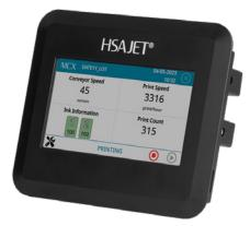
HSAJET® MCX 4.3" Touch Controller - panel mount is for use with MCX Compact Printers and MCX Satellite Printheads. It the control centre of the MCX printer from where the MCX printers are operated.
